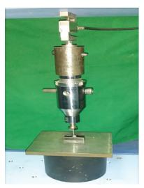
Fig. 1: Universal testing machine
